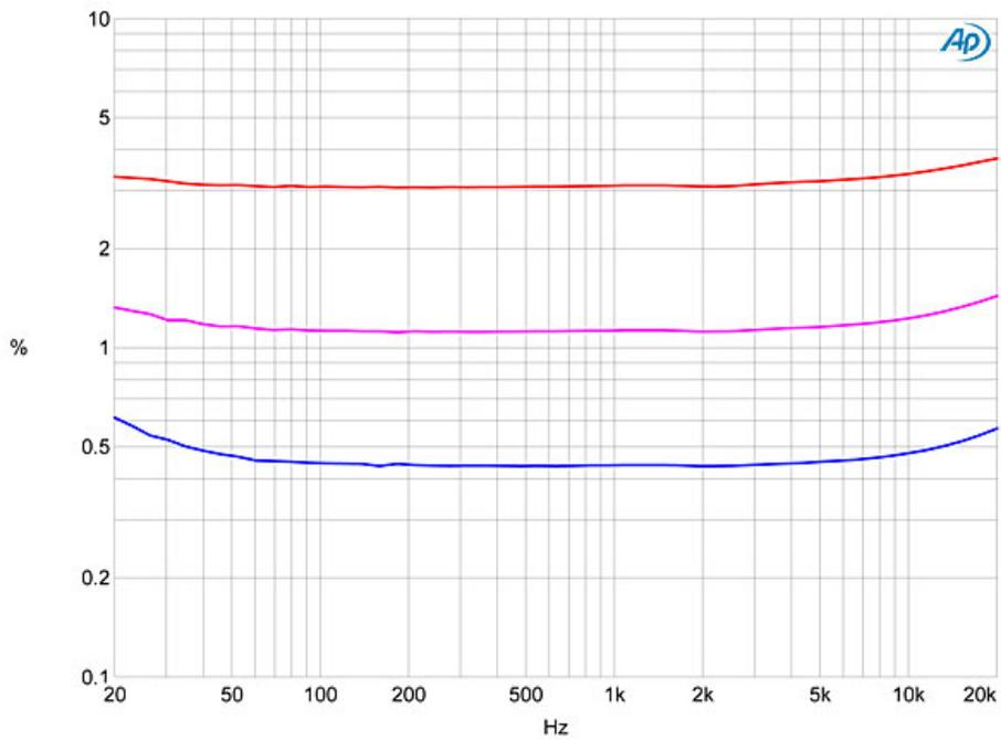
Fig.10 Lamm ML2.2, 16 ohm tap, THD+N (%) vs frequency at 2.83V into: 16 ohms (blue), 8 ohms (magenta), 4 ohms (red).
