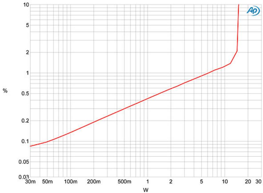
Fig.7 Lamm ML2.2, 8 ohm tap, distortion (%) vs 1kHz continuous output power into 16 ohms.
