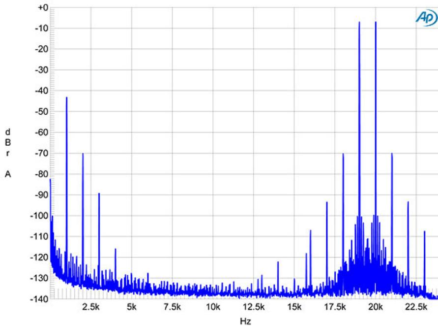
Fig.14 Lamm ML2.2, 4 ohm tap, HF intermodulation spectrum, DC–24kHz, 19+20kHz at 15W peak into 8 ohms (linear frequency scale).
