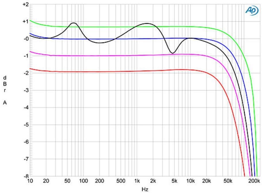
Fig.1 Lamm ML2.2, 16 ohm tap, frequency response at  $2.83\text{V}$  into: simulated loudspeaker load (gray), 16 ohms (green), 8 ohms (blue), 4 ohms (magenta), 2 ohms (red) ( $0.25\text{dB/vertical div.}$ ).
