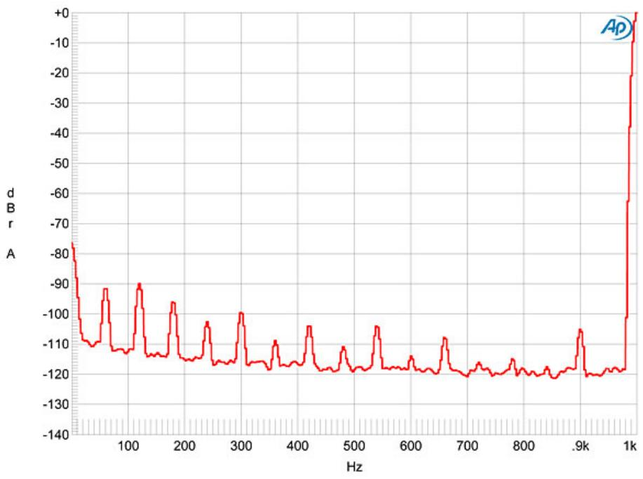
Fig.4 Lamm ML2.2, 4 ohm tap, spectrum of 1kHz sine wave, DC-1kHz, at 1W into 8 ohms (linear frequency scale).
