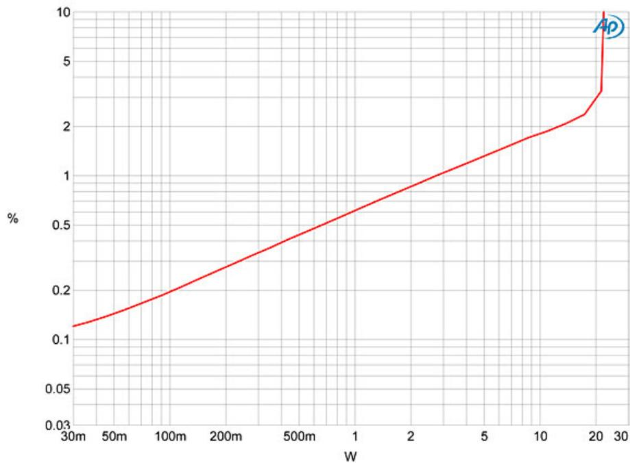
Fig.6 Lamm ML2.2, 8 ohm tap, distortion (%) vs 1kHz continuous output power into 8 ohms.
