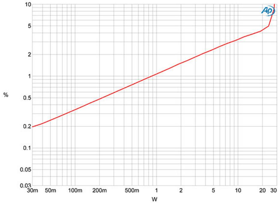
Fig.5 Lamm ML2.2, 8 ohm tap, distortion (%) vs 1kHz continuous output power into 4 ohms.
