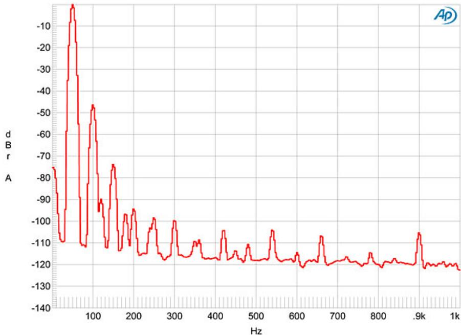
Fig.12 Lamm ML2.2, 4 ohm tap, spectrum of 50Hz sinewave, DC–10kHz, at 1W into 8 ohms (linear frequency scale).
