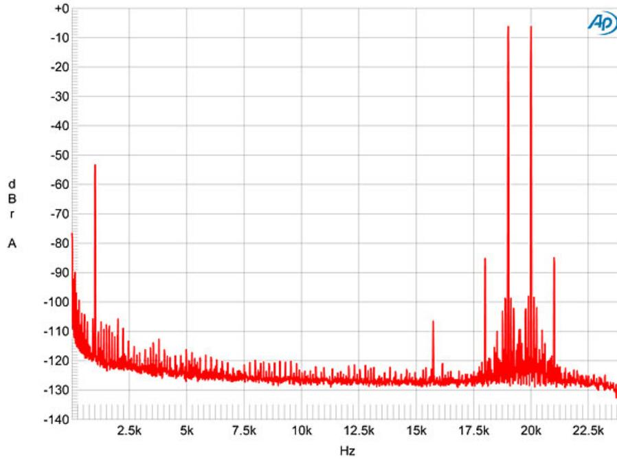
Fig.13 Lamm ML2.2, 4 ohm tap, HF intermodulation spectrum, DC–24kHz, 19+20kHz at 1W peak into 8 ohms (linear frequency scale).
