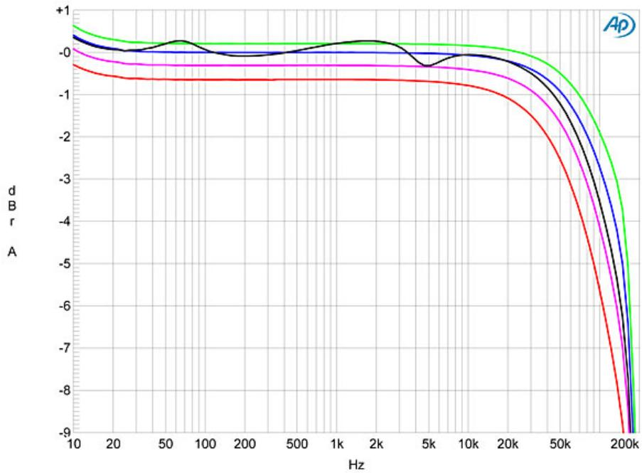
Fig.2 Lamm ML2.2, 4 ohm tap, frequency response at  $2.83\text{V}$  into: simulated loudspeaker load (gray), 16 ohms (green), 8 ohms (blue), 4 ohms (magenta), 2 ohms (red) ( $0.25\text{dB/vertical div.}$ ).
