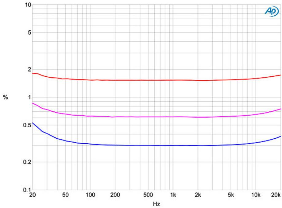
Fig.9 Lamm ML2.2, 8 ohm tap, THD+N (%) vs frequency at 2.83V into: 16 ohms (blue), 8 ohms (magenta), 4 ohms (red).
