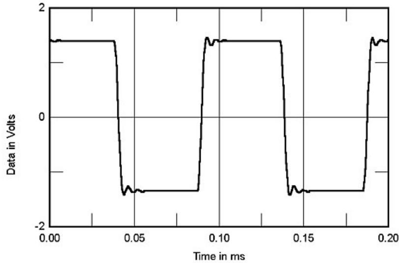
Fig.3 Lamm ML2.2, 4 ohm tap, small-signal 10kHz squarewave into 8 ohms.
