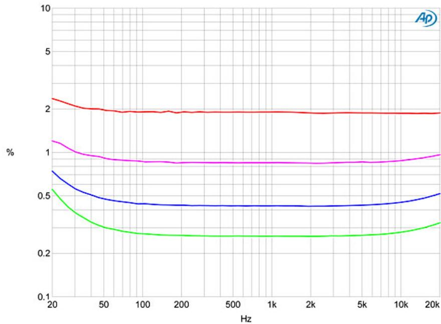
Fig.8 Lamm ML2.2, 4 ohm tap, THD+N (%) vs frequency at 2.83V into: 16 ohms (green), 8 ohms (blue), 4 ohms (magenta), 2 ohms (red).
