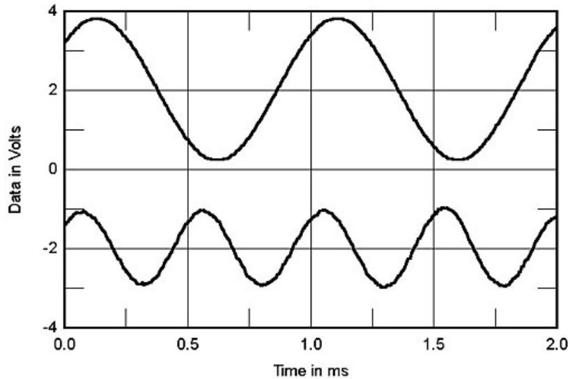
Fig.11 Lamm ML2.2, 4 ohm tap, 1kHz waveform at 1V into 8 ohms, 0.154% THD+N (top); distortion and noise waveform with fundamental notched out (bottom, not to scale).
