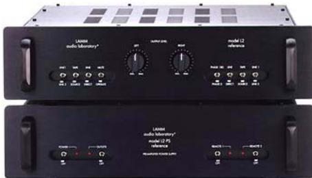
This is a two-chassis affair, with a separate power supply. Features include three RCA inputs, one tape loop, an output signal phase switch, and both balanced and single-ended outputs. The signal circuitry layout is dual monaural to minimize channel crosstalk, which explains the duplication of controls for the left and right channels, including dual TKD stepped-attenuator volume controls. There is no balance control per se; channel balance is adjustable, however, via the relative
